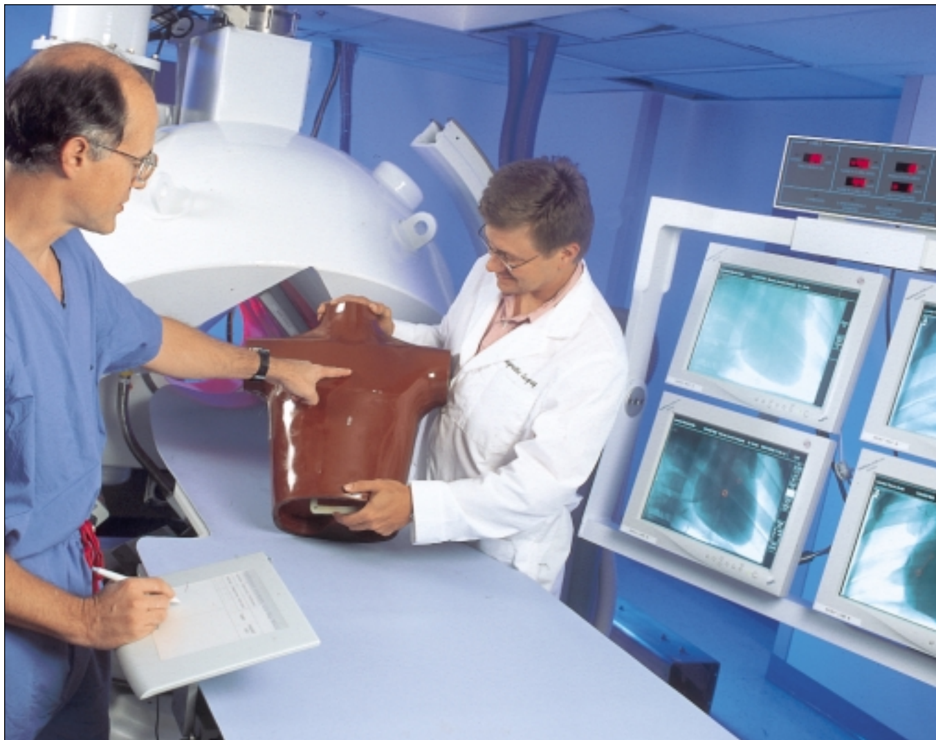
(Above) Dr. Bruce Lindsay. Dr. Bruce Lindsay (left) directs fluoroscopy calibration with a torso "phantom" to refine X-ray image quality.
